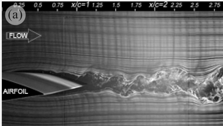
Wake downstream of an airfoil in a wind tunnel
