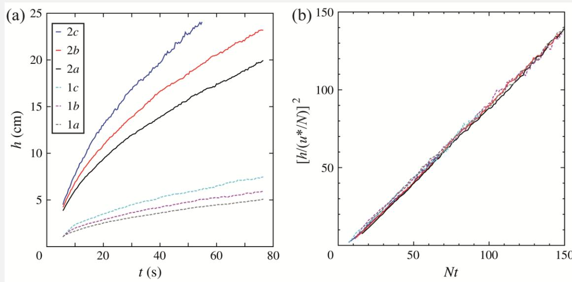
Shear-driven boundary layer growth into a linearly stratified fluid: (a) mixed layer depth evolution  $h(t)$  for six experiments and (b) collapse of data on a straight line in dimensionless form;  $N =$  buoyancy frequency and  $u^* =$  shear velocity (Jonker et al. 2013)
