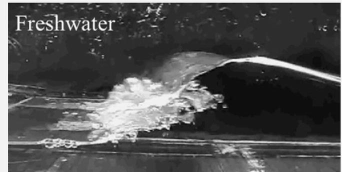
Wave breaking as an example where both F and R are relevant
