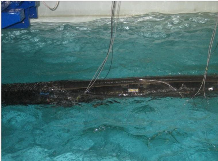
Model of Anaconda wave energy converter
