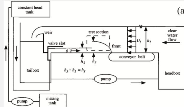
Gravity current investigated with (a) set-up based on arrested gravity current method and (b) power spectra  $G_{xx}(f)$  revealing deviations of low from high R flow data measured in most energetic region at current front (Parsons and García 1998)
