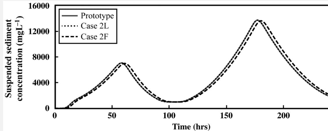
Suspended sediment concentration over time for prototype values (Prototype), for up-scaled test case based on Lie group scaling (Case 2L) and on traditional Froude modelling (Case 2F) (Carr et al. 2015)
