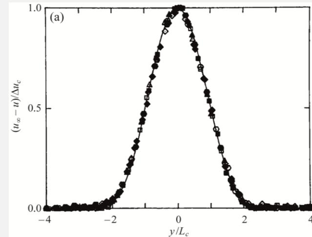
Self-similarity at solidity screen: normalised mean velocity defect versus normalised cross-flow coordinate;  $u$  = velocity,  $u_\infty$  = free stream velocity,  $\Delta u_c$  = velocity defect on centre line and  $L_c$  = distance centre line to cross-flow position  $y$  where  $0.5\Delta u_c$  (Wygnanski et al. 1986)
