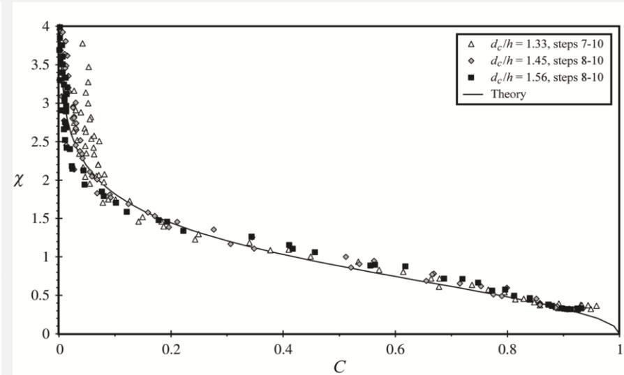
Air-water skimming flow on a stepped chute described with analytical solution (Theory): dimensionless void fraction distribution  $C(\chi)$  with  $C$  = void fraction and  $\chi$  = dimensionless parameter (Chanson and Carosi 2007)
