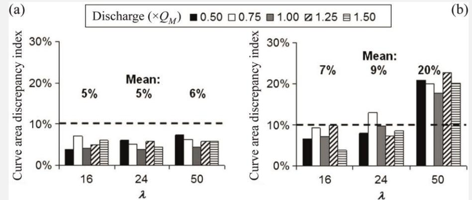
Complete mixing in a contact tank: variation of curve area discrepancy index with scale and discharge for (a) complete mixing and (b) plug flow (Teixeira and Rauen 2014)
